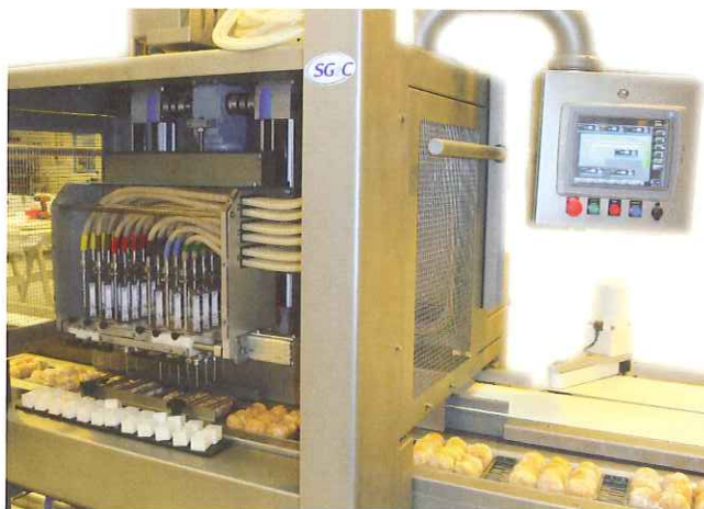
SG2C'S VERTICAL INJECTION DEPOSITING SECTION AND (BELOW) THE INTERCHANGEABLE VALVES.
